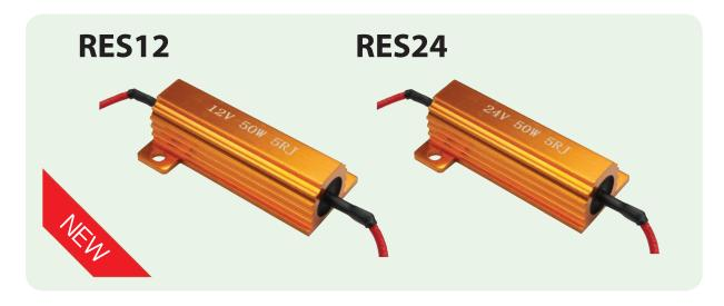
These dummy load resistors are designed to be used on vehicles that have electronic relays and components that are not compatible with LED light units. The use of this optional load resistor simulates the current draw used by a standard incandescent indicator bulb and enables the flasher unit to operate correctly. (1 Resistor per side of the vehicle)
